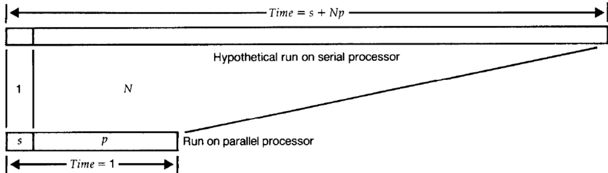
FIGURE 2b. Scaled-Sized Model for  $Speedup = s + Np$
