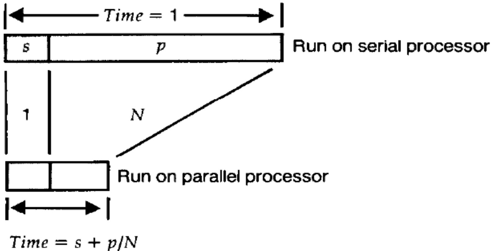
**FIGURE 2a. Fixed-Sized Model for  $Speedup = 1/(s + p/N)$**
